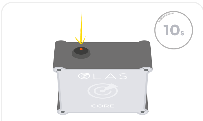
3. Cancel the alarm on the Core by pressing the control switch once. After 10 seconds the system will be tracking again.
