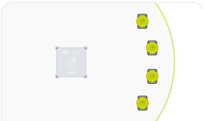
**17.** If you have other OLAS transmitters to track these can now be added to the system. Ensure all OLAS transmitters are switched on and transmitting and place them all within 1 meter of the Core.
