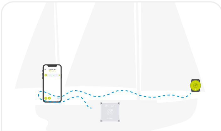
**15.** Walk around your vessel with the tag, listening out for the alarm to sound from the Core or the mobile device.
