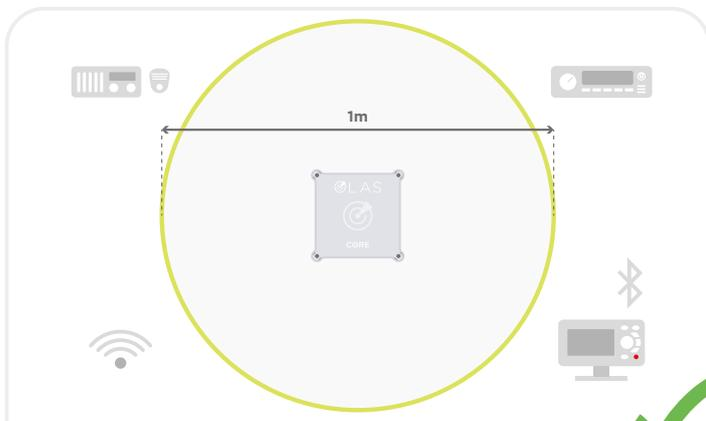
**5.** You should always try to install your Core at least 0.5 meters from any equipment transmitting radio signals including VHF Radios, antennas and cables.
