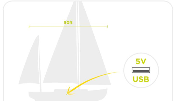
**2.** Locate a 5V USB port near the center of the vessel. Note: Power banks will not power the Core.
