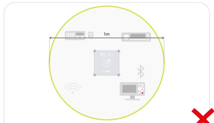
**6.** If located within 0.5 meters it is possible false alarms may occur. If you are experiencing false alarms try moving the Core hub away from other electrical devices and then carry out the Core setup and range test to see if the false alarms still occur.
