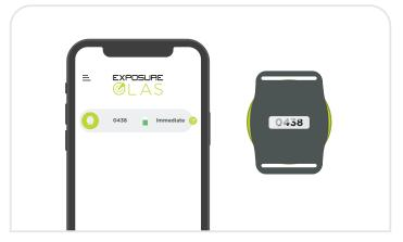
**5.** Check that the Tag displayed on the app screen has the same ID number as the Tag you are testing with. The Tag's ID number can be found on the underside of the Tag.
