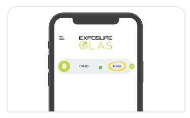
**7.** When the OLAS transmitter is up to 2 meters from the phone it should read 'Near'.
