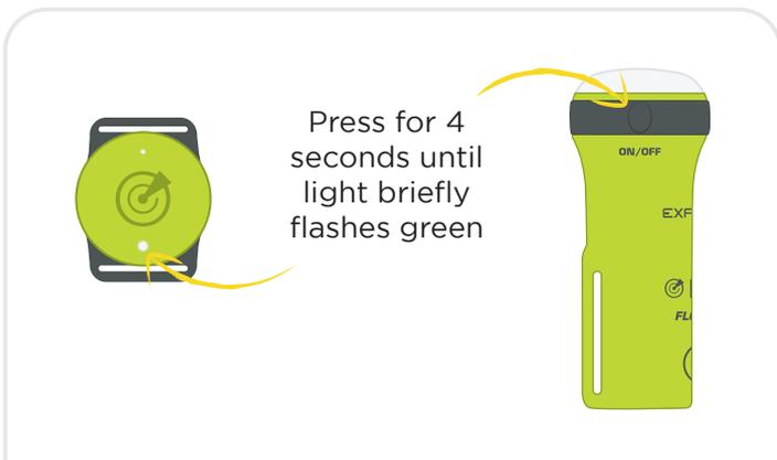
**17.** Switch the OLAS transmitter (OLAS Tag or OLAS Float-On) back on.
