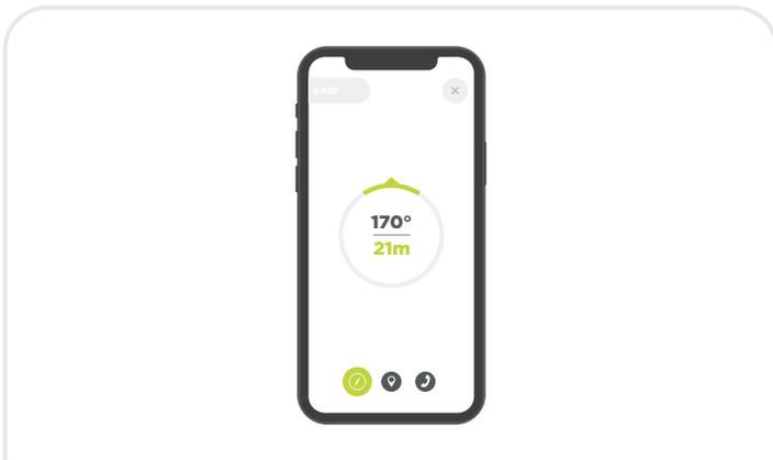
**15.** The 'Searching' screen will change to an arrow pointing back to the 'Point of loss'. It is important to note the arrow DOES NOT track the Tag, it points back to the stored GPS location where the alarm occurred, (Note: the accuracy of your GPS can vary depending on your mobile device.)
