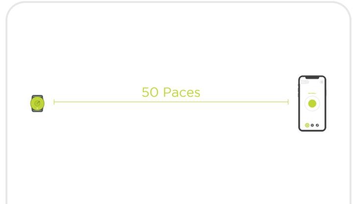
**14.** Walk at least 50 paces away from the Tag, simulating the vessel moving away from the person overboard.
