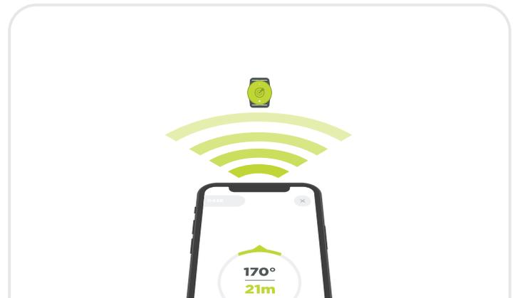
**16.** Follow the arrow towards the 'Point of loss'. This will be within the same area as the switched off OLAS transmitter. The screen will revert to 'Searching' when back within 20 meters of the 'Point of loss'.
