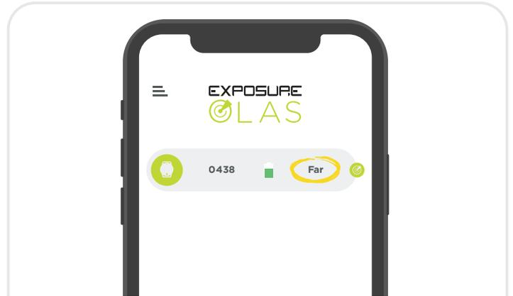
8. When the OLAS transmitter is further than 2 meters from the phone it should read 'Far'.
