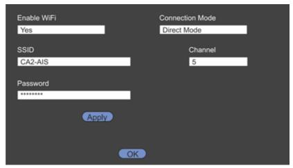
Enter the SSID to be visible to other devices, select a WiFi Channel and enter a password. **DEFAULT: SSID: CA2-AIS DEFAULT PASSWORD: ACRELECTRONICS**
