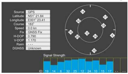
Use this page to check the quality of the internal GNSS receivers.
