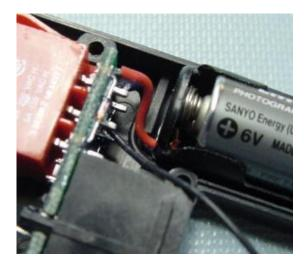
Figure 13: Conical Spring Installation
