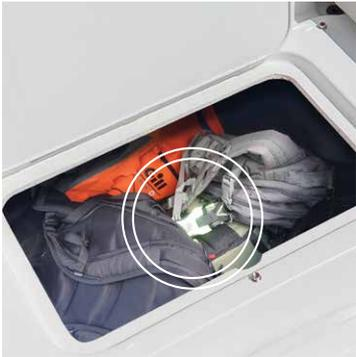
Providing ample space and not simply dropping your beacon into tight and highly compressed environments can avoid a situation where a false activation can occur.
