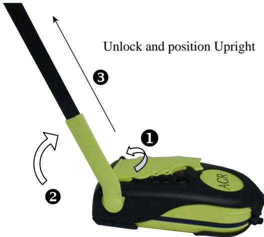
Figure 2 Antenna Position
