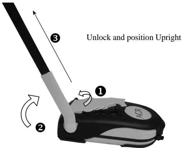
Figure 2 Antenna Position
