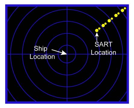
**Figure 1- Radar Distress Pattern**
