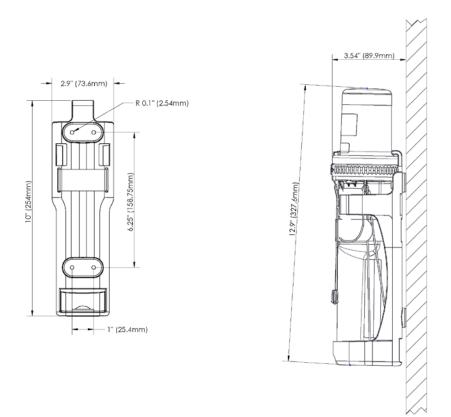
Figure 4: Installing the SART
