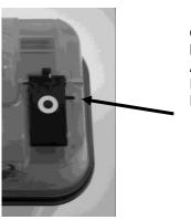
OFF position: Note the Activation Indicator Plastic Pin
