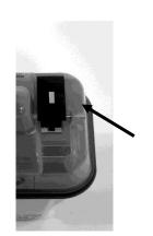
ON position: Notice the Activation Indicator Plastic Pin has been broken off.
