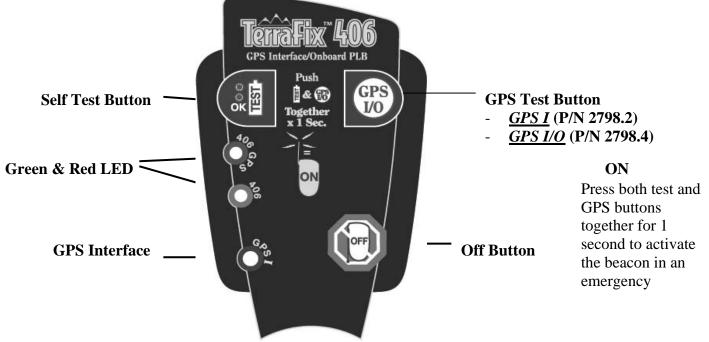
Figure 1. Key Pad Functions (P/N 2798.4 shown)
