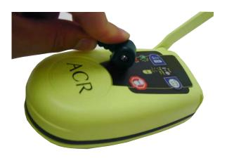
Figure 7. GPS Interface without holster
